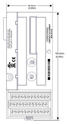
The I/O module mounts vertically (perpendicular to the DIN rail) on this carrier.
