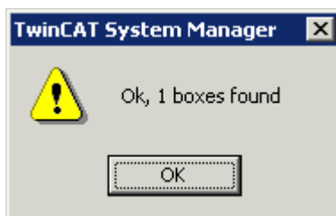
Fig. 17: The test returns the number of I/O modules (boxes) found in the ring
