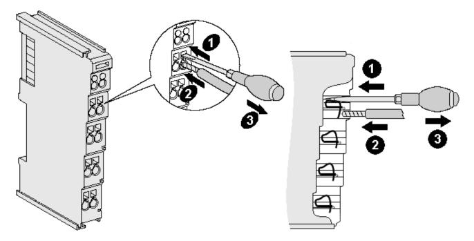
Fig. 10: Connecting a cable on a terminal point
