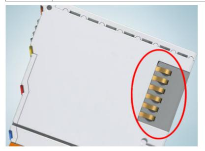
Fig. 3: Spring contacts of the Beckhoff I/O components
