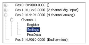
Fig. 14: KS2000 tree branches for channel 1 of the KL4494
