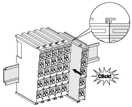
Fig. 4: Attaching on mounting rail
