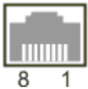
Fig. 2: Ethernet interface, pin numbering.
